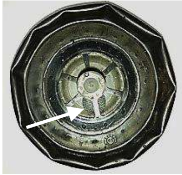
Photo 1 is a close up showing a black sizing dot (see arrow) wedged inside the facepiece regulator.
