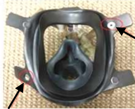
Photo 3 shows a facepiece with 2 missing sizing dots (see arrows).
