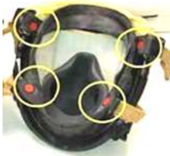
Photo 2 shows correct position of sizing dots. Sizing dots (circled) come in color-coded sets of 4.
